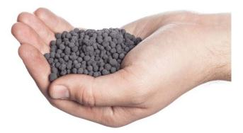
**Chlorosorb Ultra Media** has been specially engineered for use in Purafil's emergency gas scrubbers (EGS) to provide protection from a catastrophic release of
