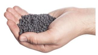
**Purafil CSO Media** has been specially engineered with a high reserve alkalinity thus assuring the best overall performance. The chemisorptive process removes contaminant gases by means of adsorption, absorption, and chemical reaction (neutralization). Harmful gases are trapped within the pellet and converted into harmless solids which remain in the pellet, eliminating the possibility of desorption and release back into the environment.
