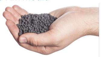
**Puracarb AM Media** has been specially engineered to provide an enhanced neutralization potential thus assuring the highest overall performance. The chemisorptive process removes contaminant gases by means of adsorption, absorption, and chemical reaction (neutralization). Harmful gases are trapped within the pellet and converted into harmless solids which remain in the pellet, eliminating the possibility of desorption and release back into the environment.
