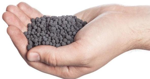
**Puracarb Media** has been specially engineered to provide an enhanced neutralization potential due to a high reserve alkalinity, thus assuring the highest overall performance. The chemisorptive process removes contaminant gases by means of adsorption, absorption, and chemical reaction (neutralization). Harmful gases are trapped within the pellet and converted into harmless solids which remain in the pellet, eliminating the possibility of desorption and release back into the environment.
