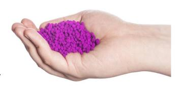
**Purafil Select Media** has been specially engineered to provide a superior oxidation potential thus assuring the highest overall performance. The chemisorptive process removes contaminant gases by means of adsorption, absorption, and chemical reaction (oxidation). Harmful gases are trapped within the pellet and converted into harmless solids which remain in the pellet, eliminating the possibility of desorption and release back into the environment.
